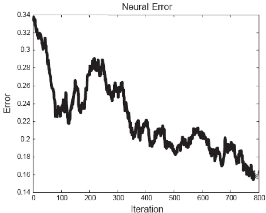
Fig.3: Training curve for the Neuro-Compensator® for 800 iterations. The error between the 'normal' and 'damaged' auditory models decreases gradually, showing how the hearing-aid amplification gain is gradually tuned to trigger proper stimuli to the brain.
