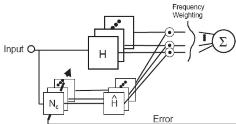
Fig.2: Block representation of the Neuro-Compensator® training sequence
